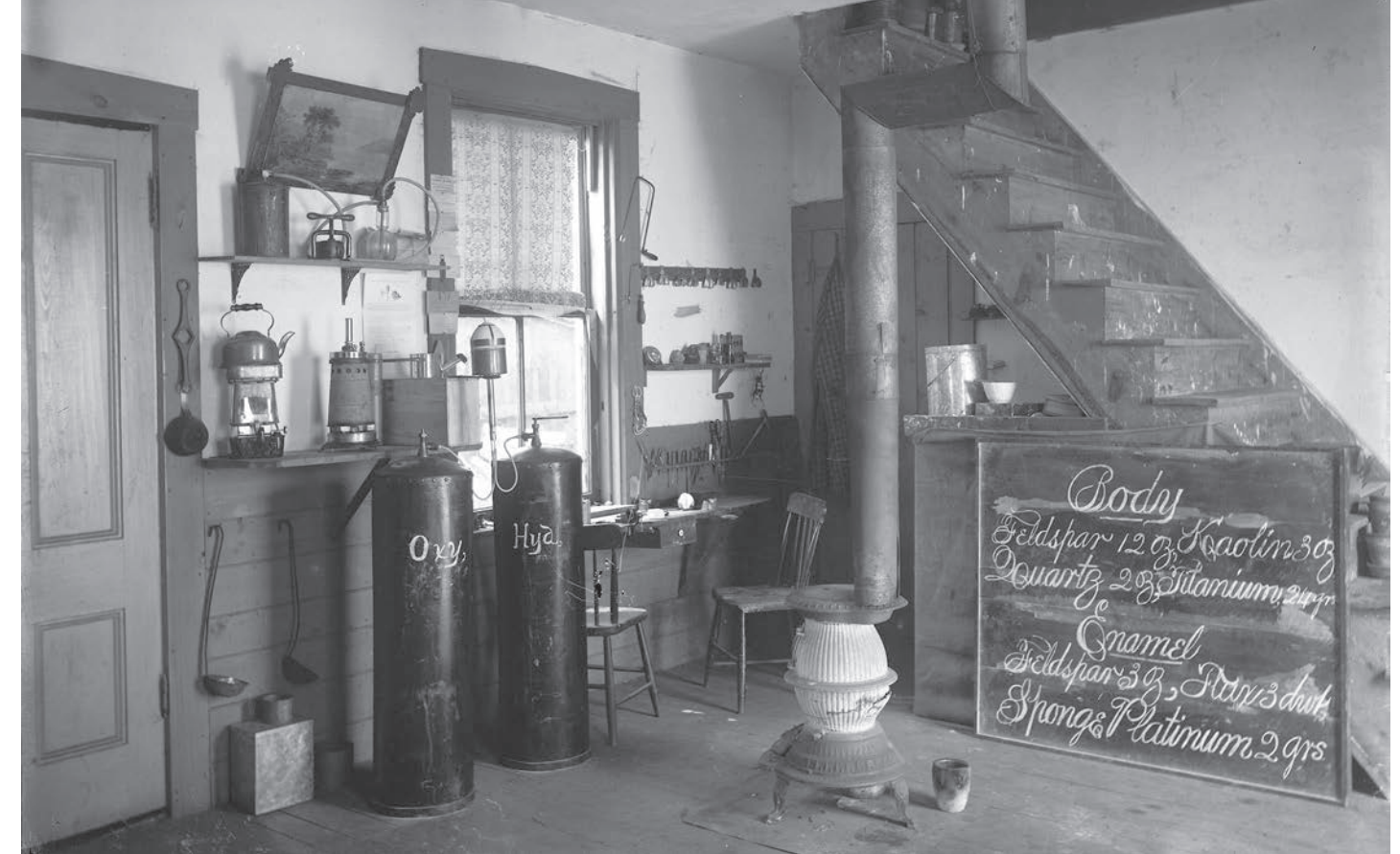
Warren M. Sharp's studio in Sussex with large, black tanks of oxygen and hydrogen being used to produce limelight for a projector. (P33-267)
